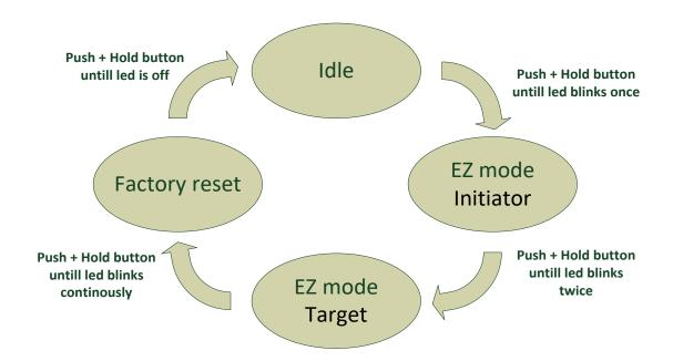
When cycling through the menu modes, the state is indicated by a number of blinks on the LED. The device is supporting the ZigBee standardized EZ- mode Commissioning.
