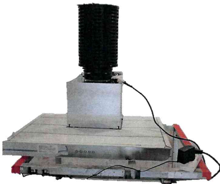
Odour filter GUC1214 with range hood in test chamber.
