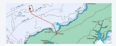
The Wave Hub site is connected to the shore via a 25 km armoured subsea cable which consists of twin 300 mm², 33 kV power triads and fibre optic cables which terminate into two isolated busbars within the the hub chamber on the seabed. Each developer will connect to hub chamber via an umbilical that will run from the lead device of each array to an 11 kV dry-mate connector on one of the Wave Hub tails.
