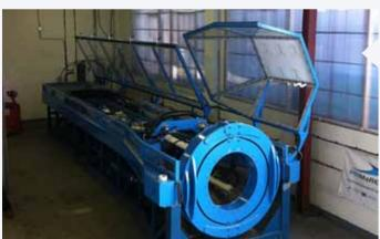
Also located in Falmouth is the custom built **Dynamic Marine Component Test Facility (DMaC)**. This one-of-a-kind rig builds upon data gathered from the SWMTF buoy to replicate the motions and forces that are applied to the component parts of marine renewable energy devices.
