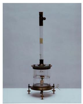
Fig. 6. Palmieri's double wire electrometer with mobile conductor. A Faraday cup collects charged ash particles. The Coulomb repulsion makes the two wires of the electrometer to detach from each other. This effect is calibrated to measure the electrostatic charge of the particles collected by the Faraday cup. This picture shows the original Palmieri instrument, which at present is at the Museum of the Osservatorio Vesuviano. With kind permission of INGV, Osservatorio Vesuviano.
