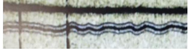
Fig. 1 The dark top line is the seismic baseline; the lower is the power grid 36th harmonic.
