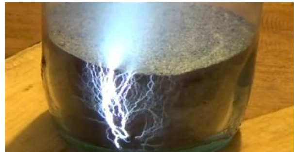
Figure 11: Electric discharge channels, slowed 8x (Gable, 2018).
