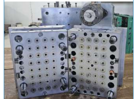
32 Cav Long Nose Temper-Proof Mould
