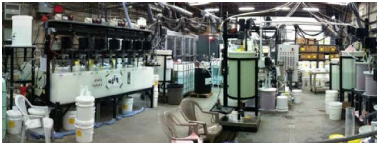
Figure 10.10 Pilot Plant (SX-Purification-Carbonation-Filtration-Washing Pulp)
