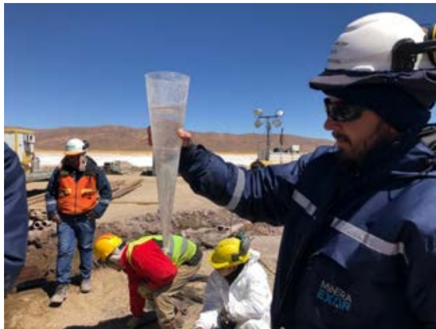
Figure 8.4 Measuring Sediment in an Imhoff Cone
