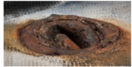
Figure 3. Post-Artemis I flight separation bolt, after the flight. Source: NASA.
