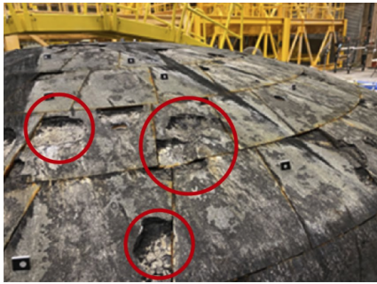
Figure 1. Artemis I heat-shield damage: heat-shield loss, including missing chunks, post Artemis I. Source: NASA.
