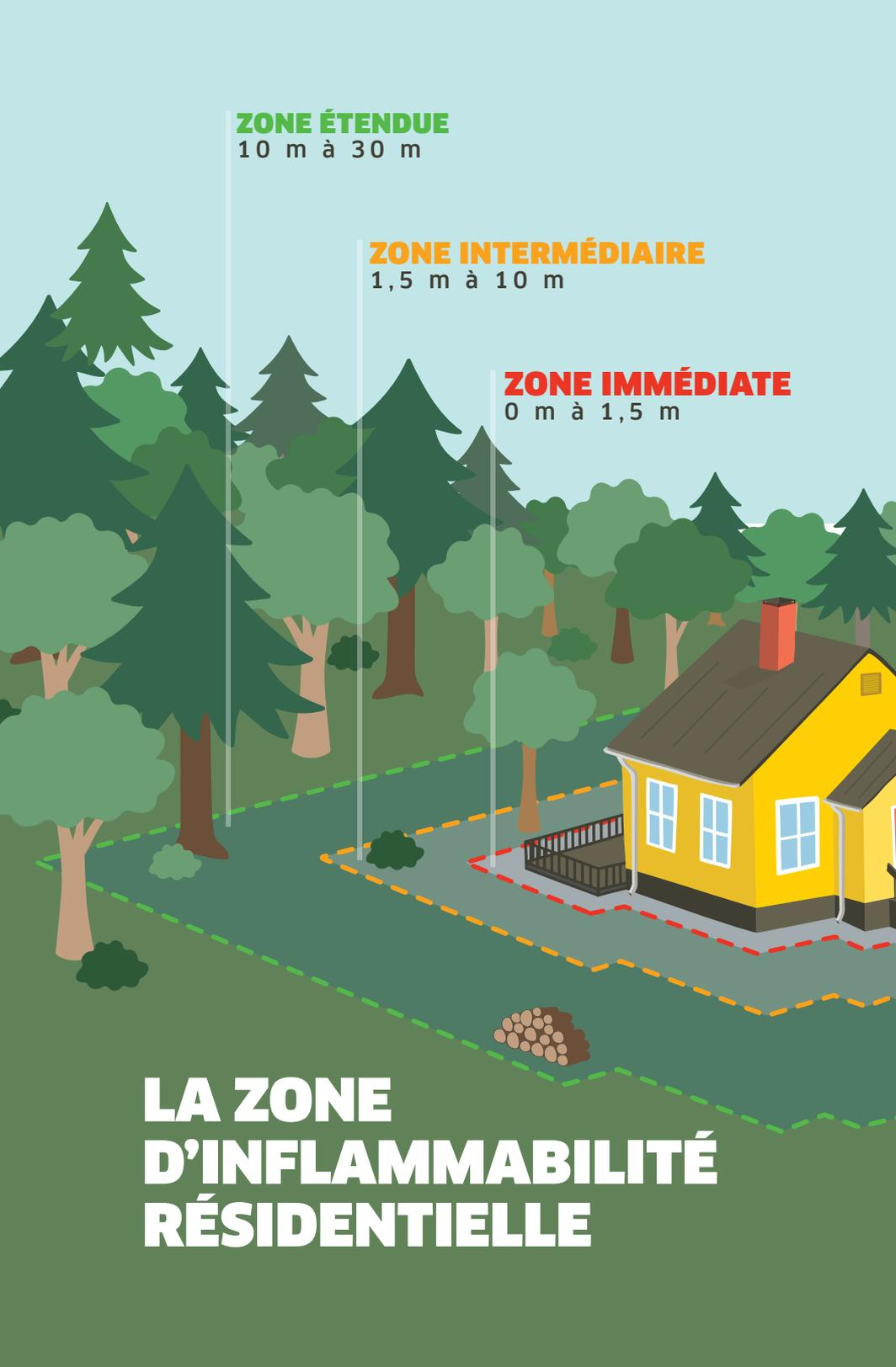
An isometric illustration of a yellow house with a brown roof and a red chimney. The house is surrounded by a forest of green trees. Three concentric dashed lines represent fire safety zones: a red dashed line (immediate zone) closest to the house, an orange dashed line (intermediate zone) in the middle, and a green dashed line (extended zone) furthest from the house. Three vertical lines indicate the distances between these zones. A pile of logs is shown in the foreground.
