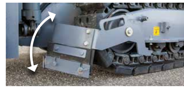
4 Raise/lower deflectors in front of the crawler tracks
