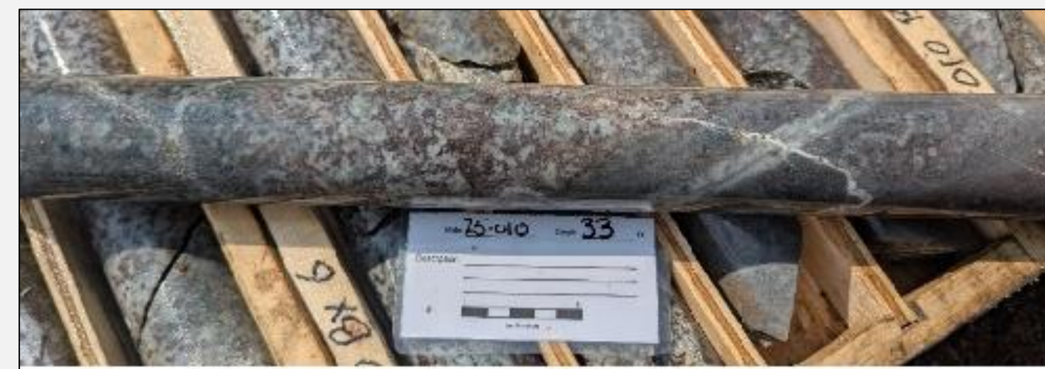
ALT-25-010 at 33 m - Quartz-sulphide veins developed within strongly altered granodiorite from the south Severance Zone.
