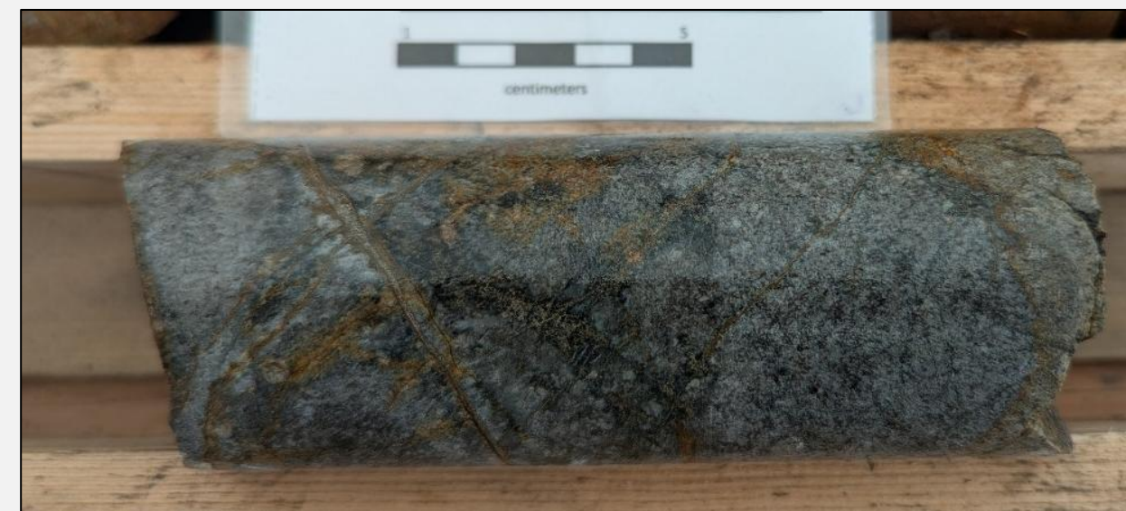
ALT-25-007 at 1.8 m - Oxidized quartz-pyrite veins alongside biotite altered quartz feldspar porphyry
