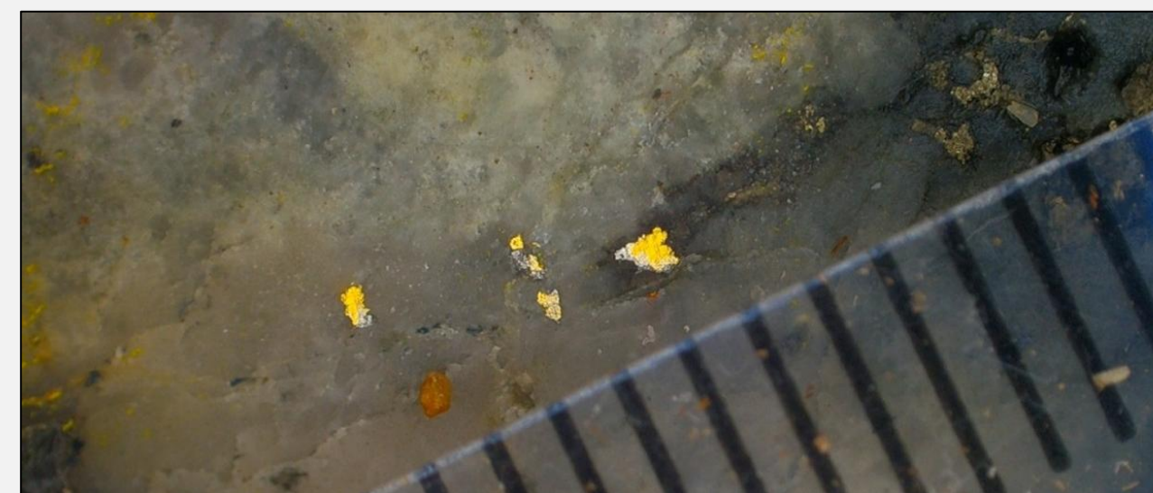
ALT-25-008 at 56 m – Quartz vein hosting visible gold
