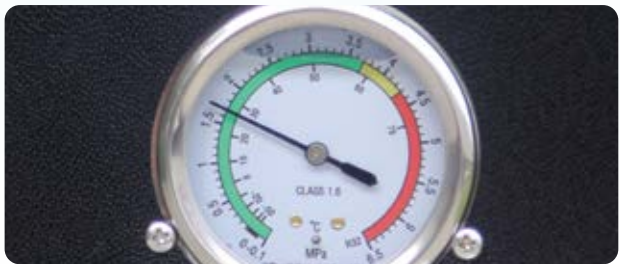
Refrigerant System Pressure Gauge
