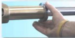
Insert the new bearing on the shaft. We recommend to use Caravel bearings, thanks to the quality of their materials and the perfect tolerances with the puller-fitter tools.
