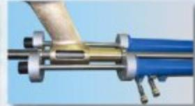
Insert the "A" ring in the flange which is between the end of the shaft (now without propeller) and the strut. Insert the half-rings ("semi-anelli") in the other flange (which is between the strut and the hull). The puller-fitter is now anchored to the shaft.
