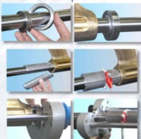
Connect the clutches of the puller-fitter to the pump.
