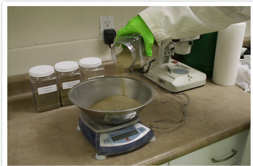
Figure 3: Recombination of classified aggregate to create sample aggregate
