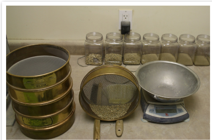
Figure 2: Gradation and classification of decomposed granite aggregate
