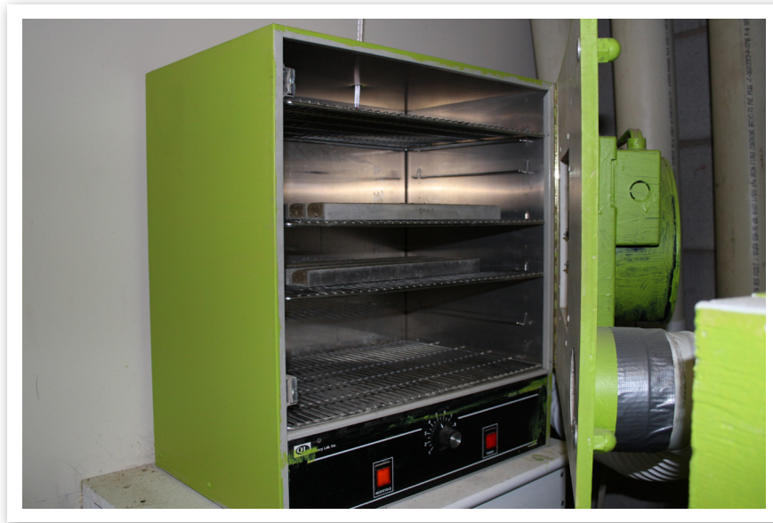
Figure 7: Rainfall simulator samples being placed in incubator for natural drying
