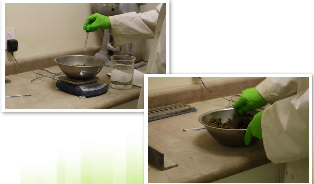
Figure 5: Dry sample material mixed by hand with water.
