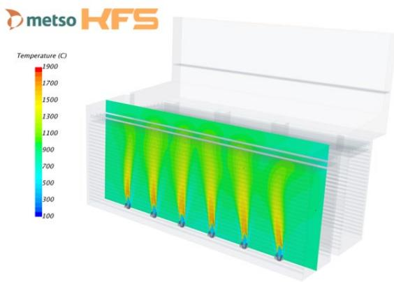
Our 3D CAD system provides real-time control over burner design changes identified through CFD simulation. It allows us to generate detailed modification drawings and implementation plans if modifications are required in order to overcome constraints in existing systems.
