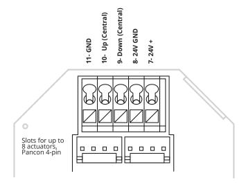
Figure 2: Connection designation (front, upper half of the housing)
