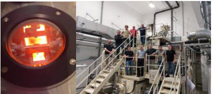
Vacuum Induction tests to produce pure Dysprosium performed in the U.S.
