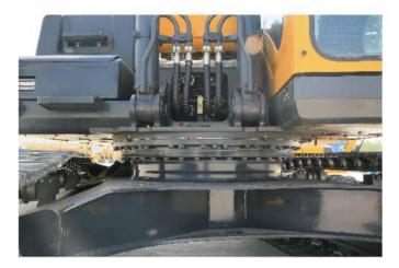
Adopt the Finite Element Analysis (FMA) to strengthen the key parts of the boom and arm. Use the new type of shaft locking mode and increase the plate thickness. The arm has the regeneration function, which can fully improve the operation efficiency, coordination and stability of the whole machine.
