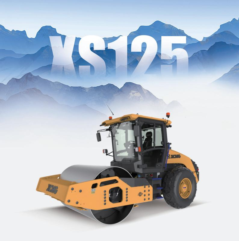
XS125 single drum roller is medium, self-propelled, full-hydraulic vibratory roller, has the big exciting force, high compaction efficiency, good compaction quality, used mainly for compaction operation of base coarse, sub-base coarse, stone filling of high-speed railway, high-grade highway, airport, harbor, dams and industrial construction site.
