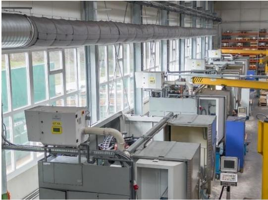
Figure 4: Processing machines with self-cleaning oil/emulsion mist filters with Hepa filters and recirculation mode
