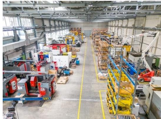
Figure 7: Machine hall with heat dissipation and machine extraction systems with oil/emulsion mist filter
