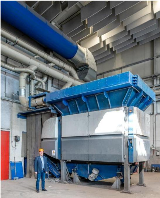
Figure 6: Shredder with attached extraction ring and associated exhaust air piping and draught-free air recirculation
