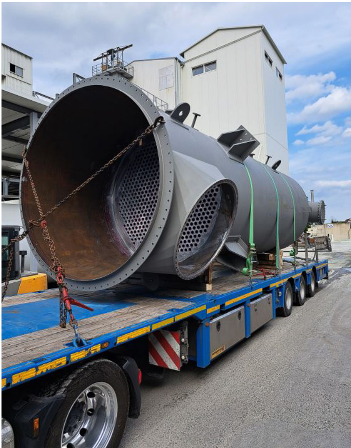
Image 05: Delivery of the new heat exchanger. An important step in optimizing energy efficiency.
