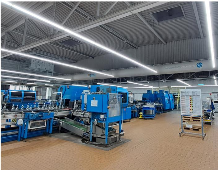
**Image 04:** The textile supply air hose system ensures a draft-free and even distribution of the conditioned air.
