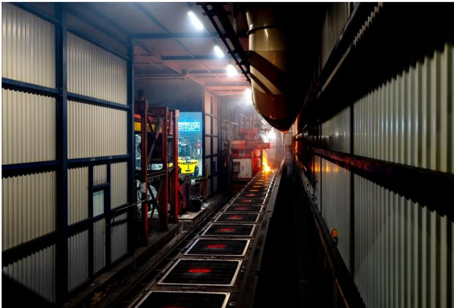
Enclosure of the casting line with zone-controlled extraction
