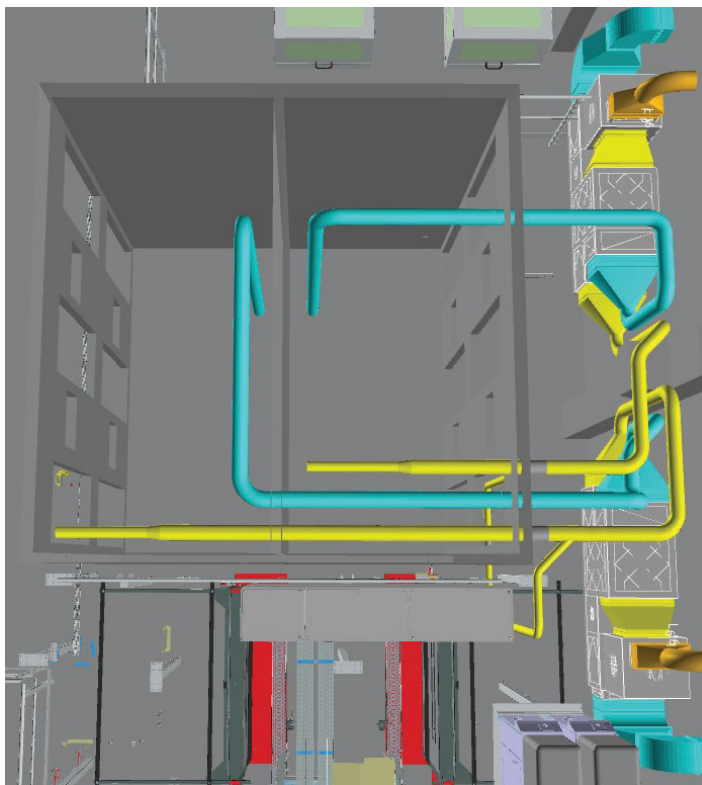
Picture 01 and 02: 3D visualization of the heat recovery system for the paper drying lines at IBS Austria
