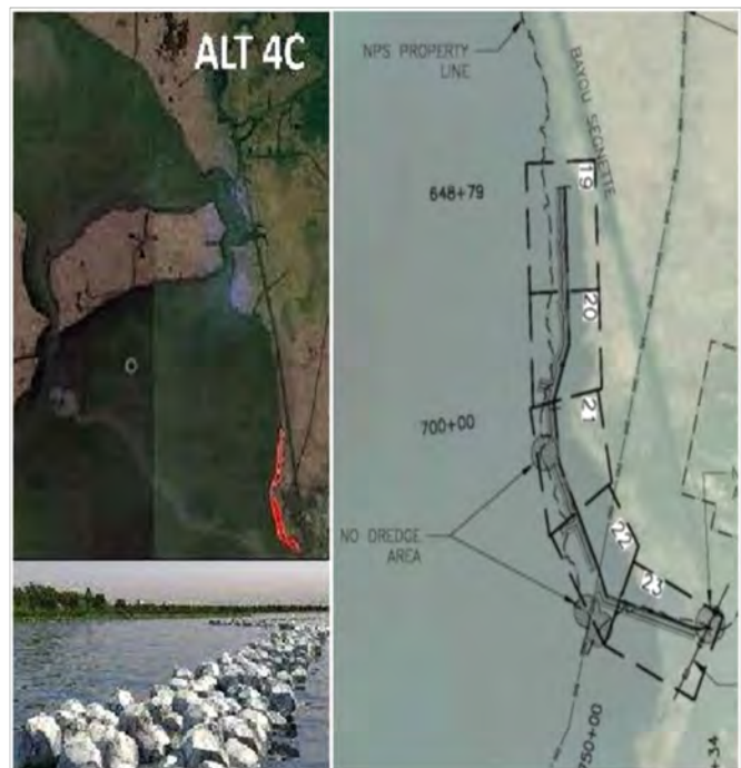
Rock breakwaters on the southern portion of Lake Salvador for the Jean Lafitte Project. Courtesy of LA TIG.
