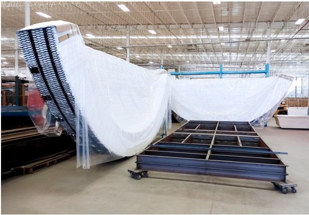
Fig. 3 This melter roof was constructed in three sections to facilitate shipment and assembly
