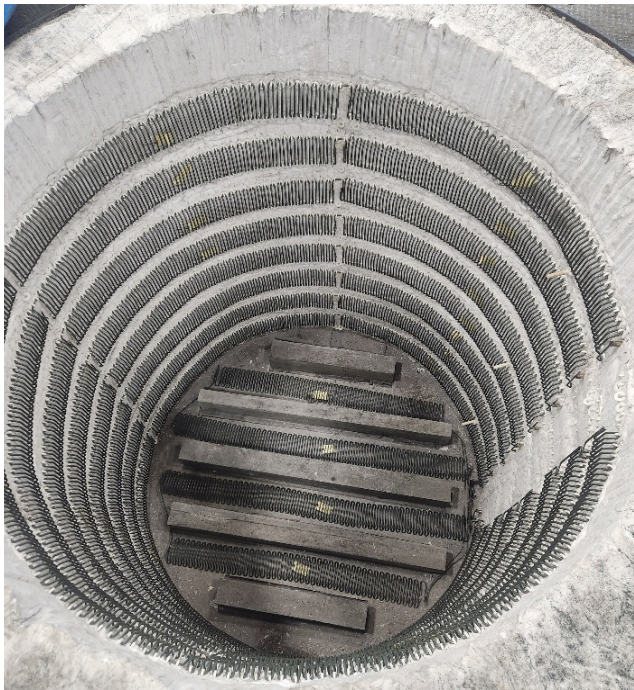
Fig.3 MaxBlock Element Module Pit Furnace
