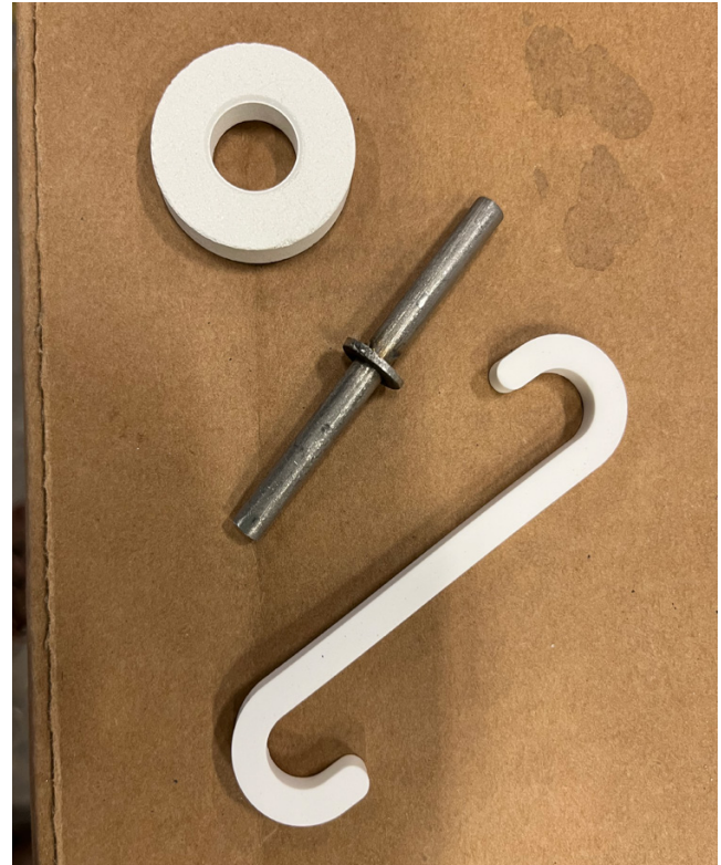
Fig. 2 Alignment Pin, Hook and Washer
