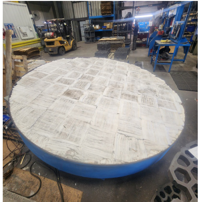
Fig.4 MaxBlock Module Pit Furnace Cover
