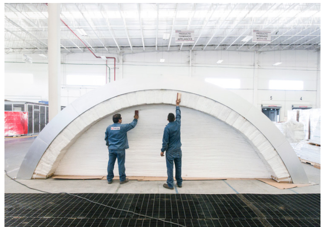
Fig. 3 MaxBlock MacroModules - Panelized Roof Construction
