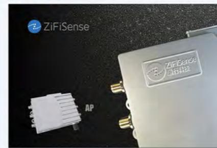
The AP is a bridge relaying data between end-devices and ZETA Server in the backend. AP connects to end-devices via ZETA protocol while connects to ZETA Server via standard IP connections. All connections support bi-directional transmission, and support unicast, multicast and broadcast to target devices.
