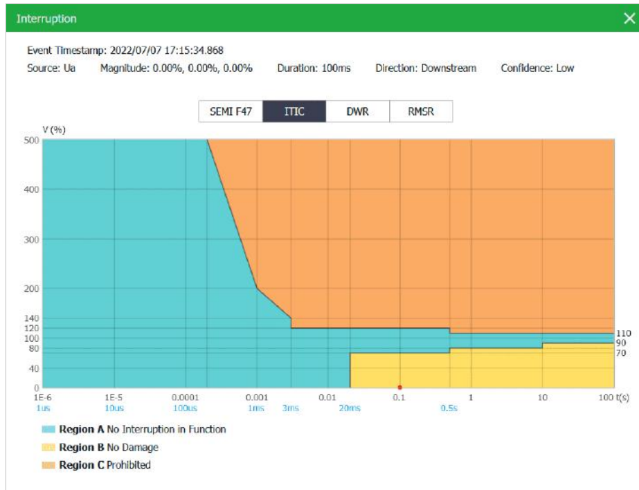
Figure 3-101 Interruption on ITIC Interface
