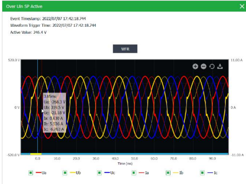
Figure 3-99 Over Uln Setpoint Active
