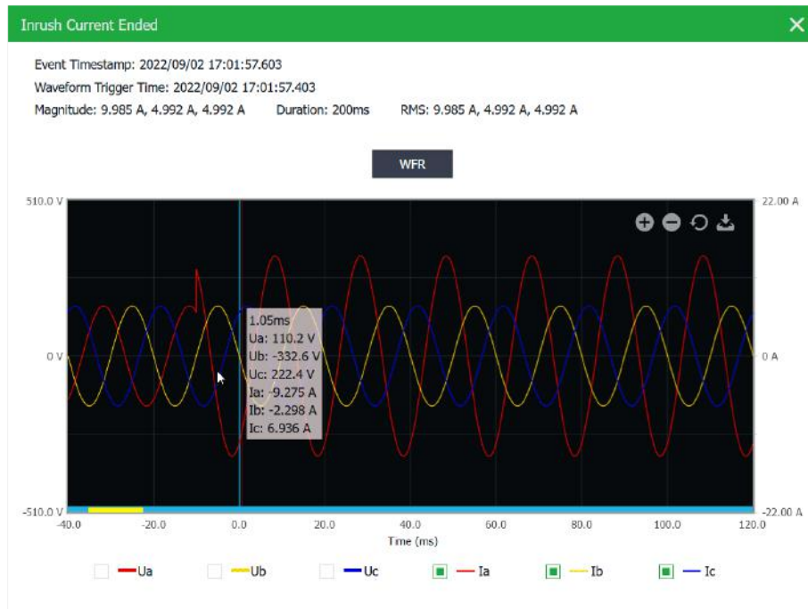
Figure 4-18 Inrush Current - displayed on Web Server
