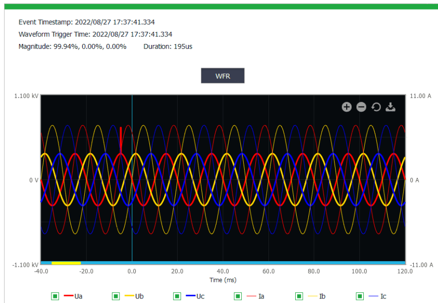
Figure 4-11 Transient Event @ 512 samples/cycle x 100 cycles
