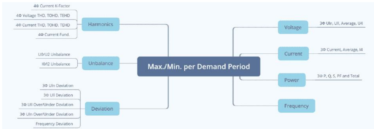
Figure 4-26 Max./Min. Parameters per Demand Period
