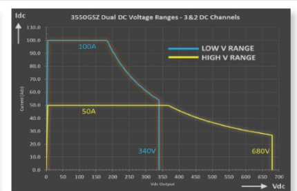
Figure 2: High and Low DC Voltage Ranges - Current vs. Voltage - 55kW
