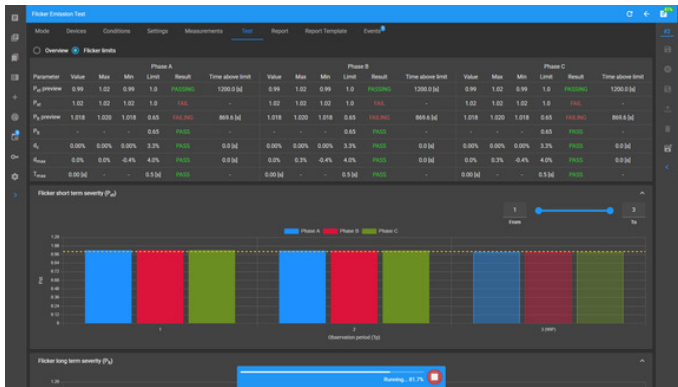
Flicker-Pst Limits and Short Term Graph Measured Flicker readings for each phase with Pst charts
