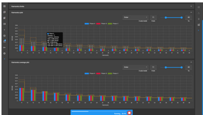
Harmonics - Voltage Limits Check Table run 4.5% Example of a Fail result for source Vthd
