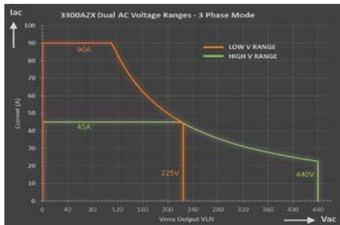
Figure 3: High and Low AC Voltage Ranges - Current vs. Voltage - 30kW
