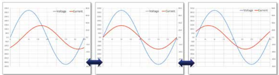
Programmable Current Phase Shift for Power Factor Control
