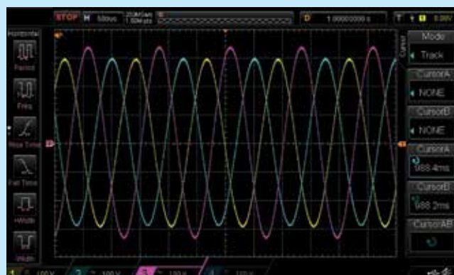
Three Phase Unbalance Voltage Test Captured
