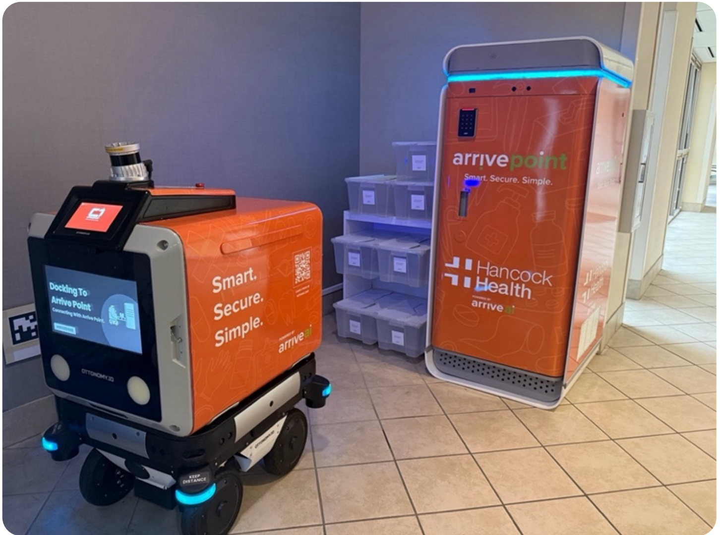
Figure 4. Blue LED light indicating that the Arrive Point™ has an item inside it which the Ottobot will pick up.
