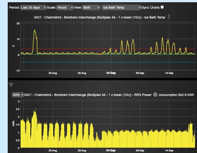
0421 Chelmsford – Power fluctuation affecting ice bath temperature
