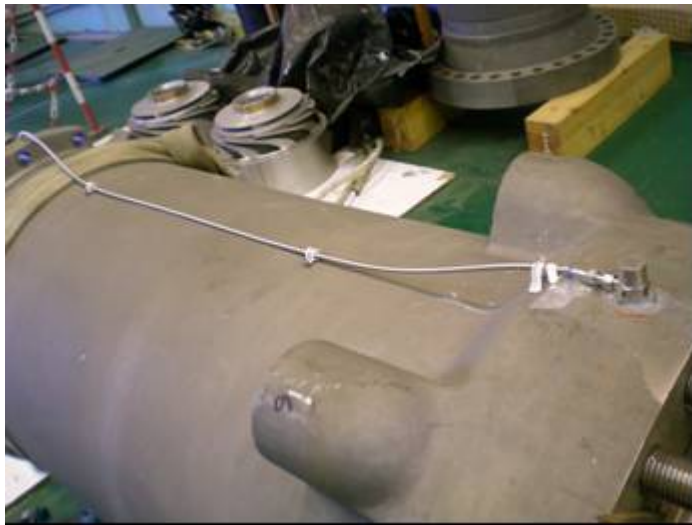
Figure 3.- Accelerometer directly attached to the LNG pump (an ex-tank pump in this case). Accelerometer in contact with LNG.
