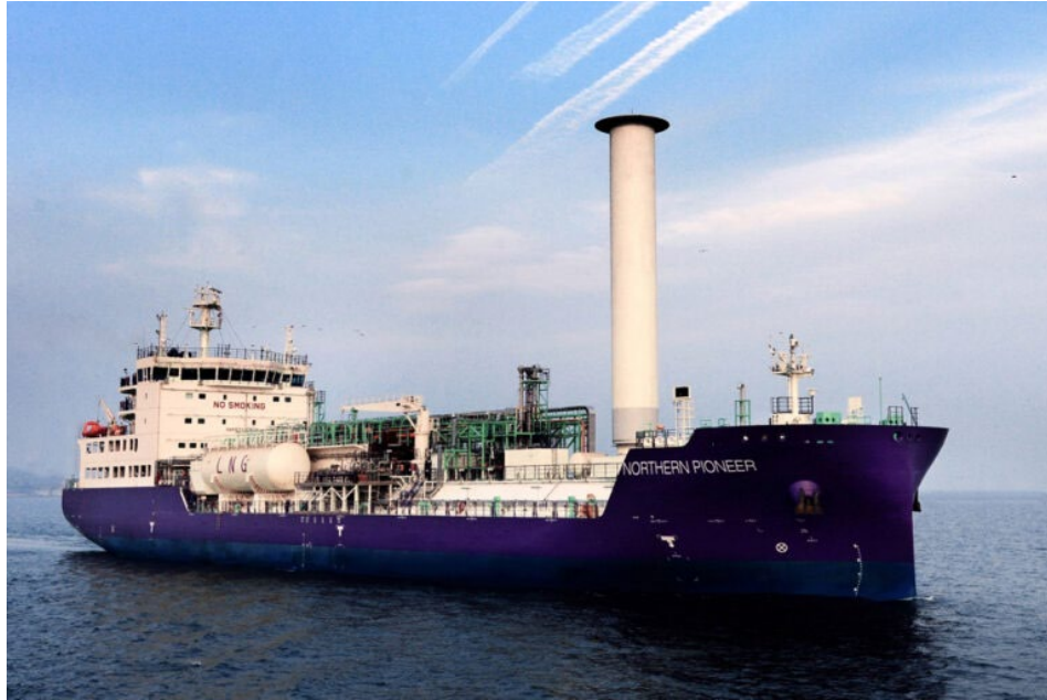
Figure 4 – Northern Pioneer - 7,5 k cbm CO 2 carrier (Credit: K Line)
