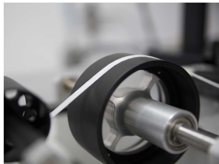
Ex: low tension web system is needed for low tensile strength materials
