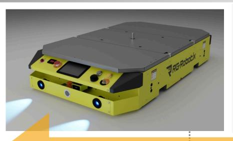
The Big Buddy is a dual direction AGV is designed to enhance operational efficiency with its advanced maneuverability and robust safety features. This AGV is adept at handling intersections and navigating complex pathways, thanks to its ability to turn in place and smoothly process tape crosses.
