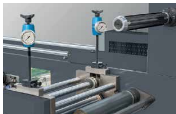
Die Cutting Unit with Matrix Rewind
