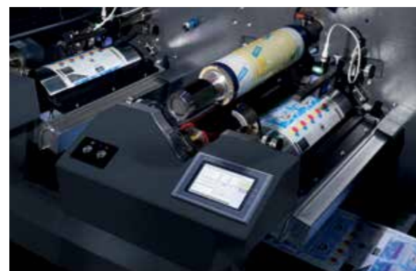
Sleeve system with three servo motors
