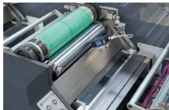
Flexo Print Unit with Gear Cylinder (Single Servo)
