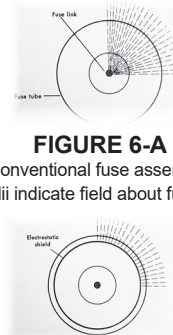
FIGURE 6-B Southern States shielded tube showing transfer of field away from link
