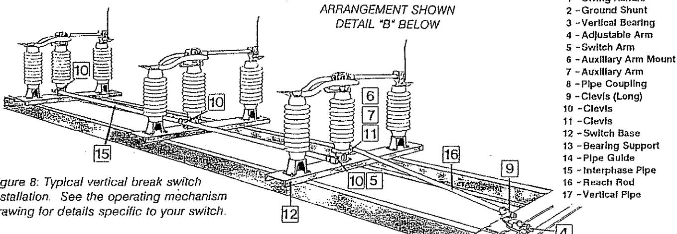
Figure 8: Typical vertical break switch installation. See the operating mechanism drawing for details specific to your switch.
