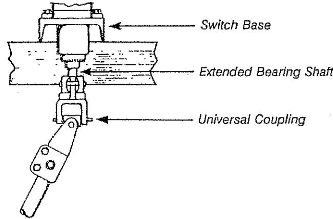
Figure 12: Vertical pipe attachment to the universal coupling
