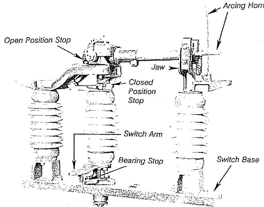
Figure 1: Identification of parts (EV 34.5 kV shown)
