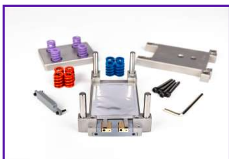
Fig. 2 - Setup assembled for tests under the "fixed force" protocol (left), with the jig equipped with pressurizing springs. Charge and discharge profiles, along with the stabilized force response that actively compensates for cell swelling, are shown on the right.
