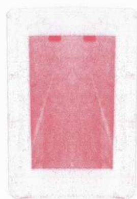
Pressure distribution on a pouch cell sample using pressure pads
