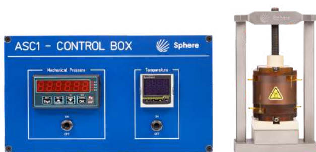
ASC CONTROL BOX with pressure frame and ASC-T+ cell
