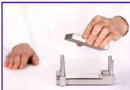
Fig. 1 - Setup assembled for tests under the "fixed thickness" protocol (left), where the plates are locked in place after applying the desired pressurizing force. Charge and discharge profiles, along with the force response to cell swelling, are shown on the right.
