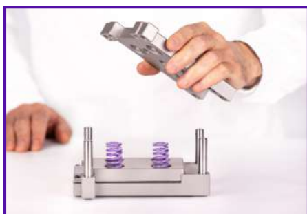
Fig. 2 - Setup assembled for tests under the "fixed force" protocol (left), with the jig equipped with pressurizing springs. Charge and discharge profiles, along with the stabilized force response that actively compensates for cell swelling, are shown on the right.
