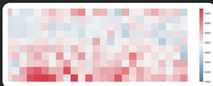
Pressure map of a pouch cell. High- and low-force zones, followed through cycling.
