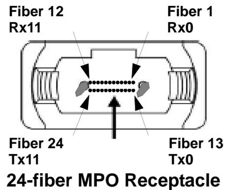
**Rotated 24-fiber MPO Receptacle, e.g., for below-PCB mounting**
