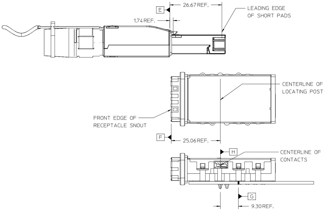
**Figure 6 Cable Connector and Receptacle Housing Datums**
