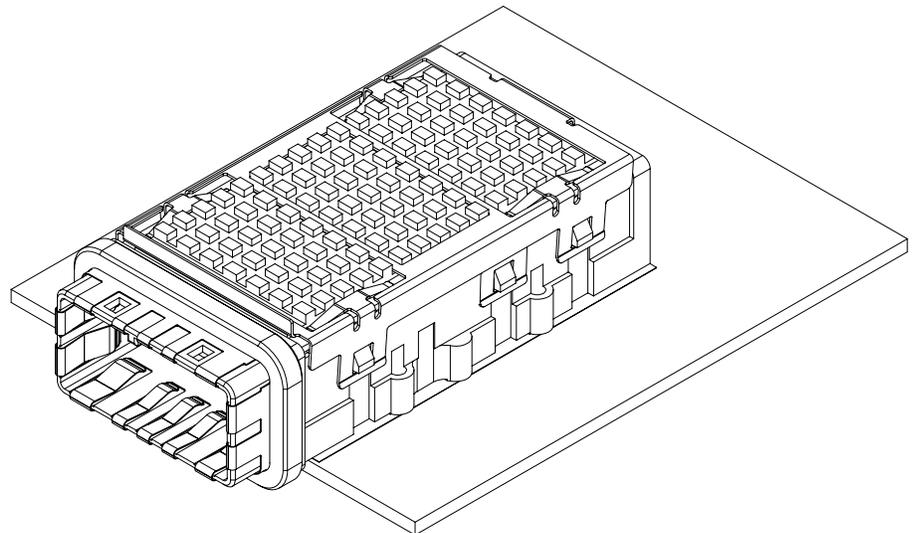
**Figure 16 Receptacle Housing with Integrated Riding Heat Sink**
