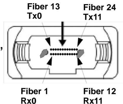
**Figure 27 Connector orientation for 24-fiber MPO/MTP connector**
