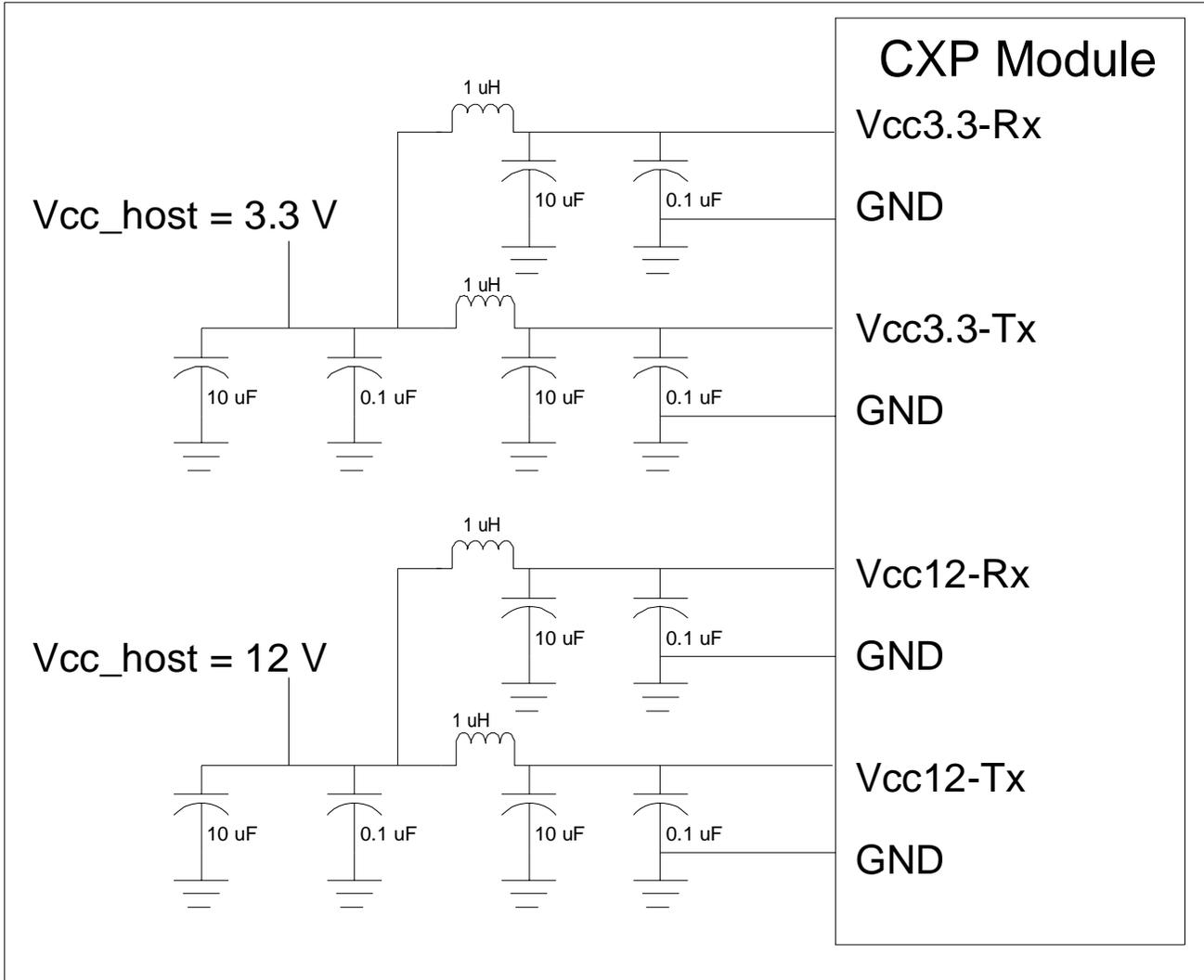
**Figure 3 Recommended Host Board Power Supply Filtering**
