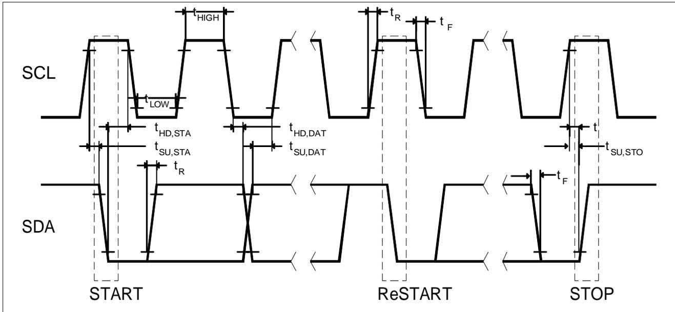
Figure 29 CXP 2-wire Serial Interface Timing Diagram
