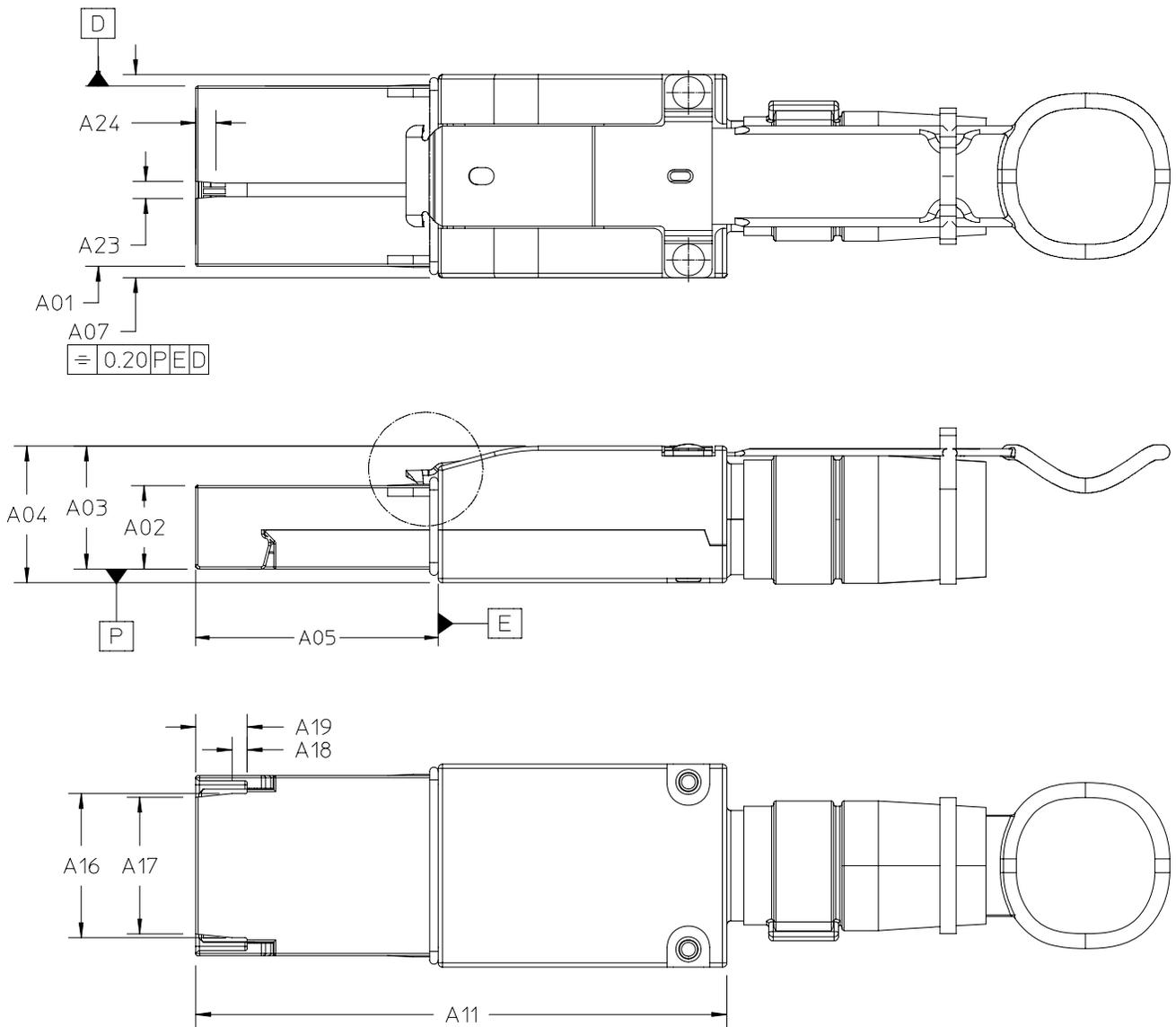
**Figure 7 Shielded Free (Plug) Integrated Cable Connector**
