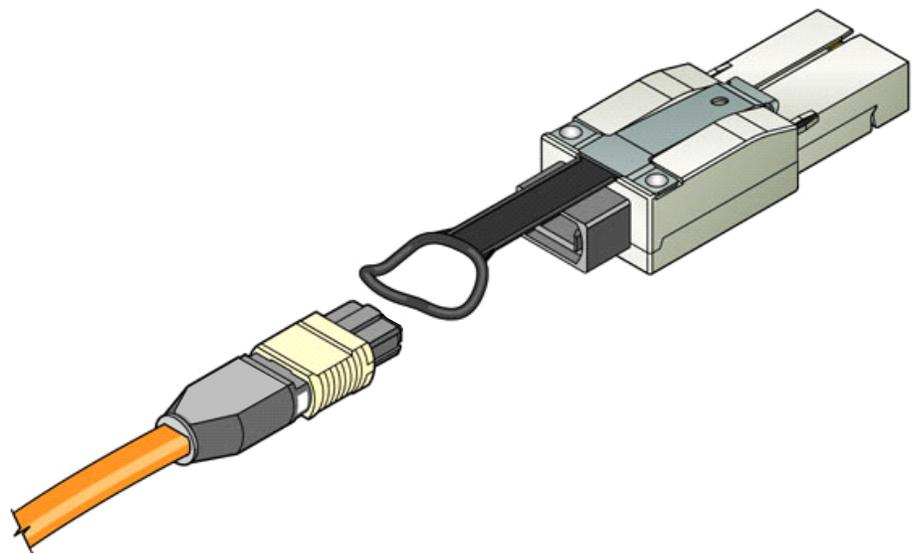
**Figure 22 Optical Transceiver with separable optical cable**
