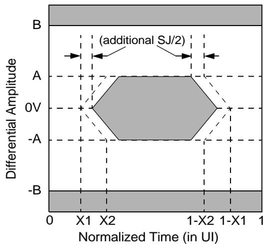
**Figure 42 – Deriving the tolerance mask at the interoperability T points**
