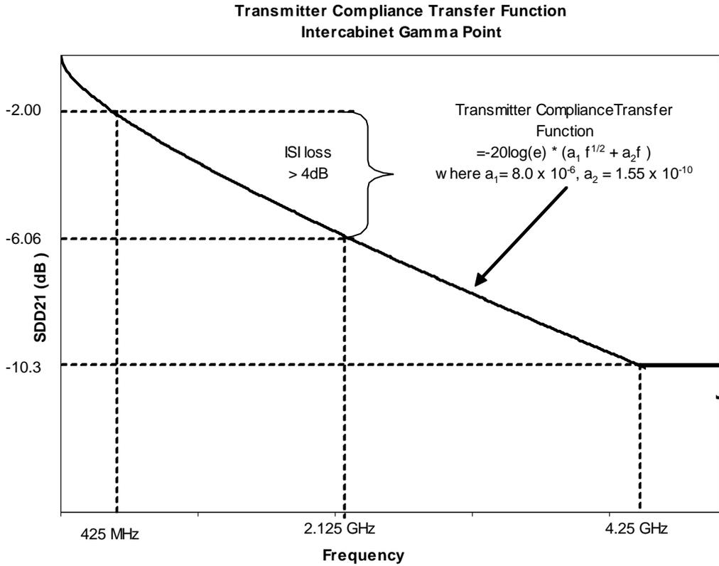
**Figure 51 – 400-DF-EL-S Inter-enclosure transmitter compliance transfer**
