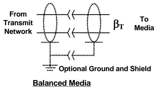
Figure 48 – Intra-enclosure transmitter compliance point  $\beta_T$
