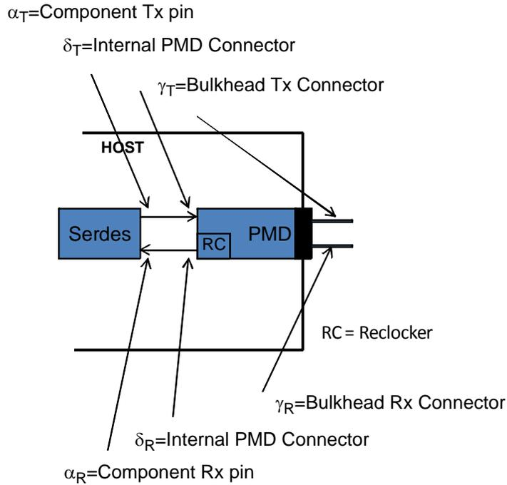
**Figure 7 – reclocker location for 1600-SM-LC-L and 1600-SM-LZ-I**
