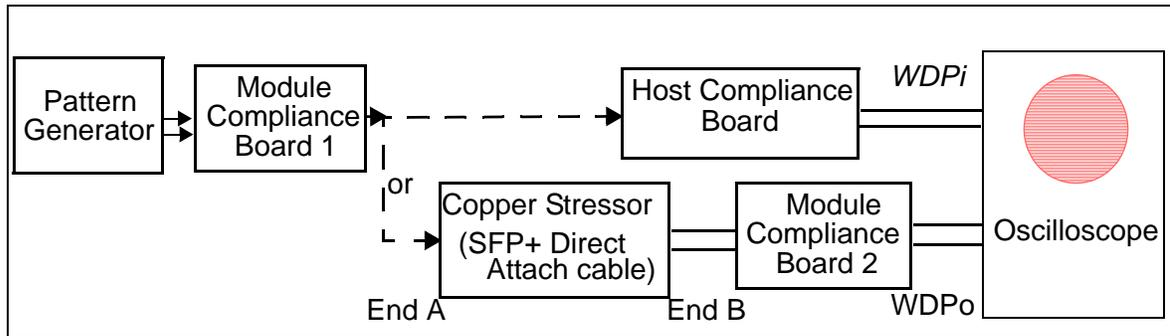
**Figure C.4 – SFP+ direct attach cable NEXT dWDP test setup**
