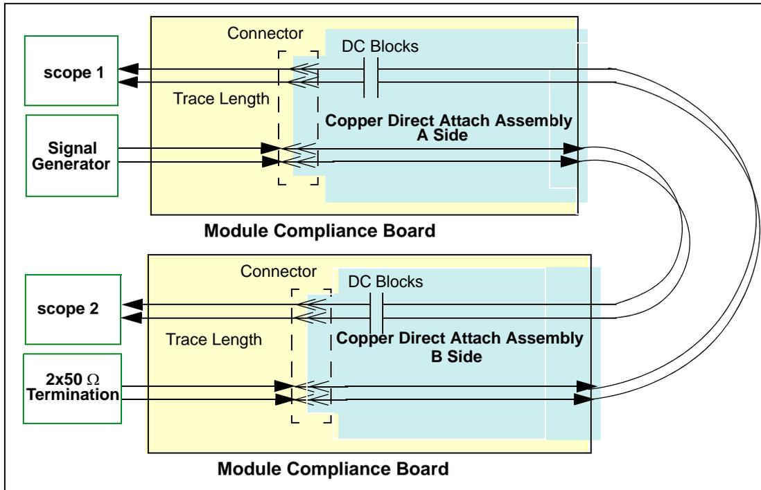
**Figure C.3 – SFP+ direct attach cable measurement**
