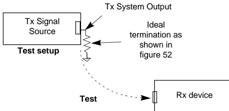
**Figure 36 – Signal tolerance test set up for Rx device at delta R**
