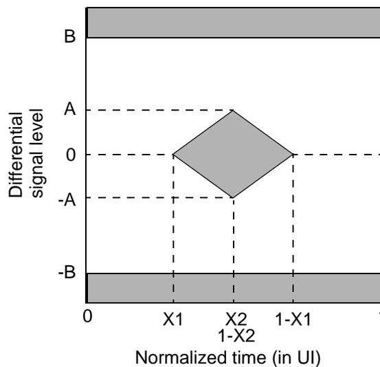
**Figure 41 – Eye diagram mask at  $\beta_R$ ,  $\delta_R$ , and  $\gamma_R$  for EL variants**
