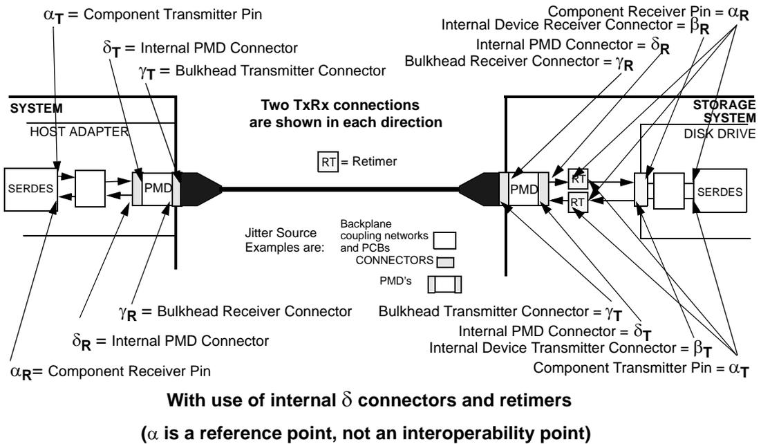
**Figure 11 – Interoperability points examples at connectors**
