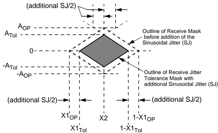
**Figure 43 – Deriving the tolerance mask at the interoperability R points**
