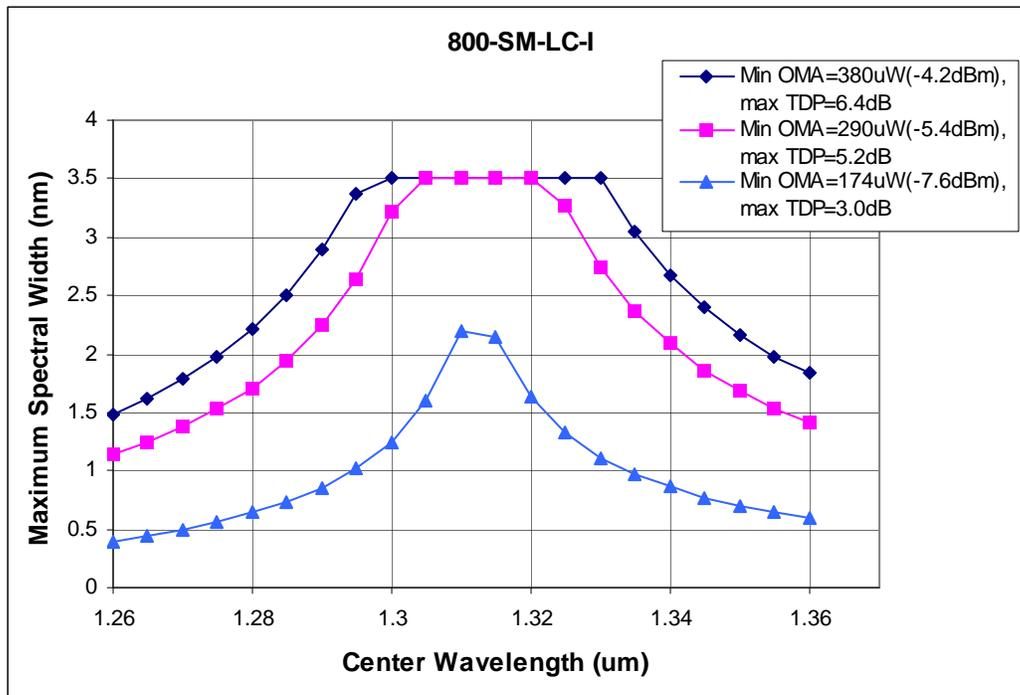
Figure 25 – 8GFC SM 1.4 km link
