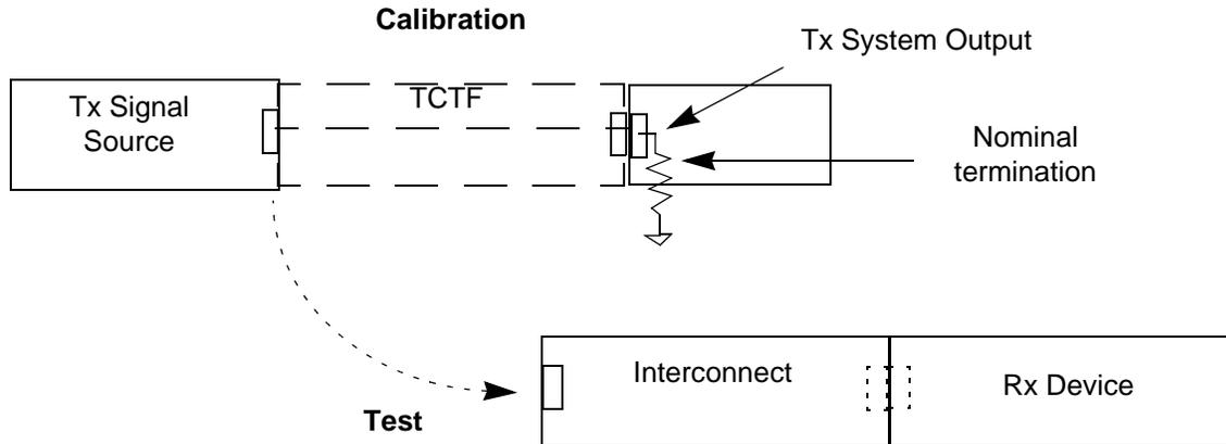
**Figure 31 – Transmit, system (interconnect + receiver device) input tolerance test**
