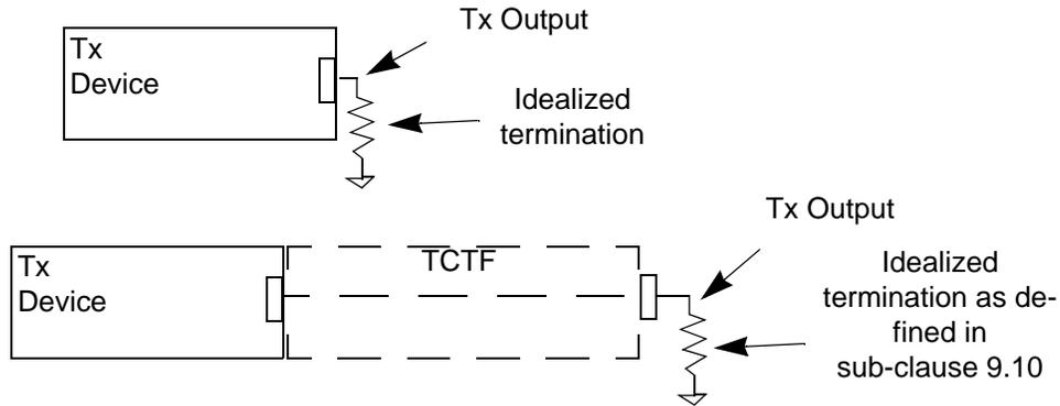
Figure 30 – Transmit device output, Zero length and through TCTF
