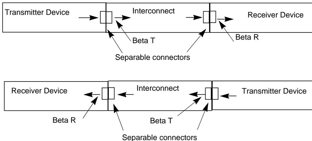
**Figure 17 – Duplex beta TxRx connections example**
