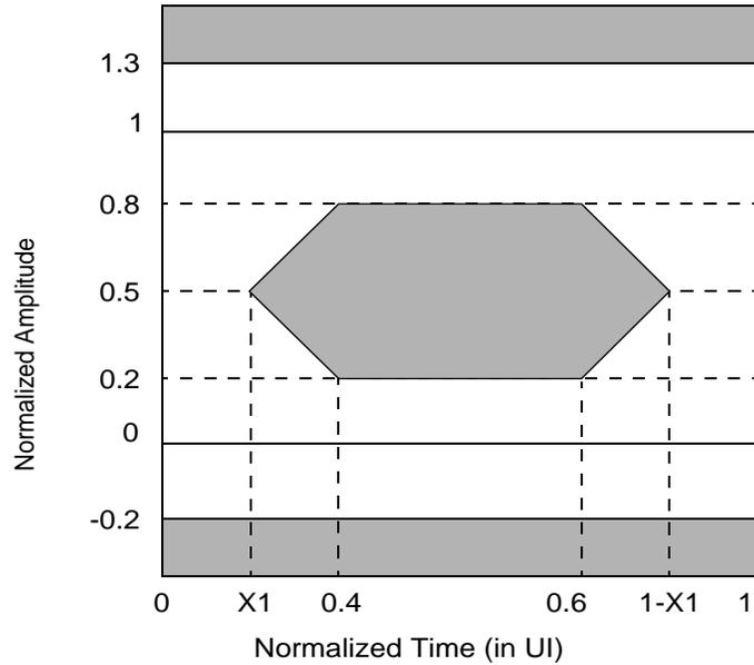
Figure 26 – MM transmitter eye mask for 4GFC
