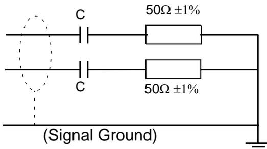
NOTE: Capacitors are required if output under test is not DC isolated. Value of C is 100 nF for 16GFC and 10 nF for 8GFC and 4GFC.
