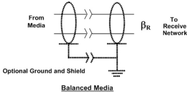
Figure 49 – Intra-enclosure receiver compliance point  $\beta_R$
