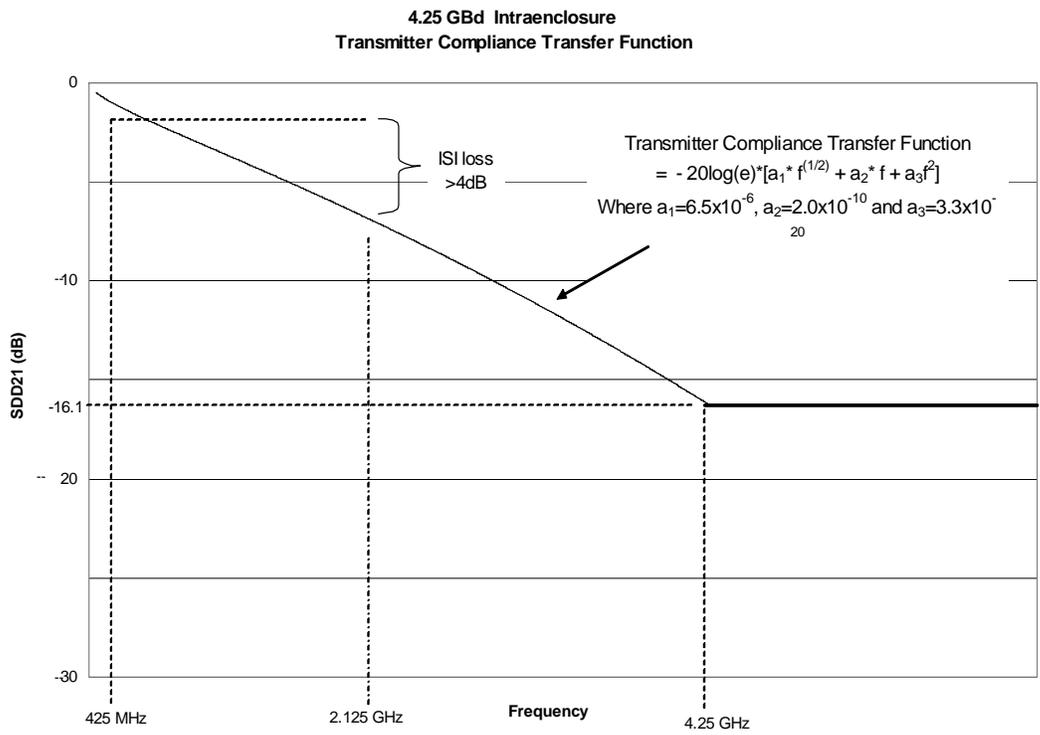
**Figure 50 – 400-DF-EL-S Intra-enclosure Transmitter Compliance Transfer Function**
