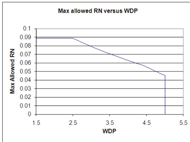
**Figure D.2 – Trade-off between RN and WDP for 800-DF-EA-S delta R**
