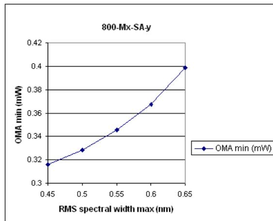
**Figure D.1 – RMS spectral width and OMA trade offs**
