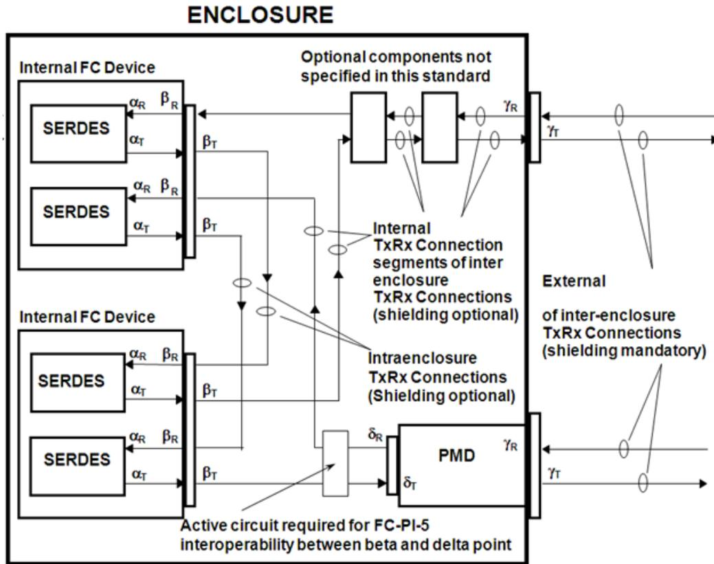
Figure 10 – Example of physical location of reference and interoperability points
