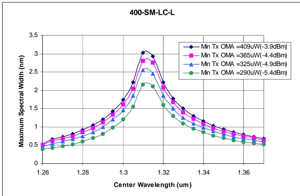
**Figure 23 – 4GFC SM 10 km link**
