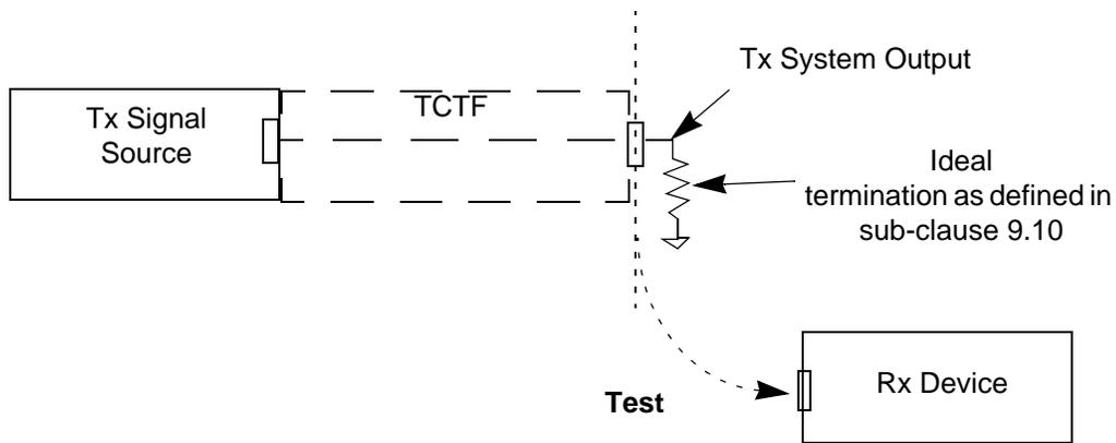
**Figure 35 – Signal tolerance test set up for Rx device at beta R and gamma R**
