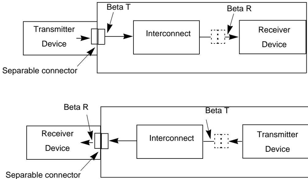
**Figure 19 – Partially Separable links examples**
