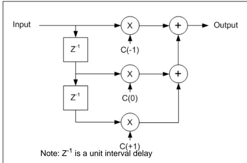
**Figure 46 – Transmit device equalizer function model**
