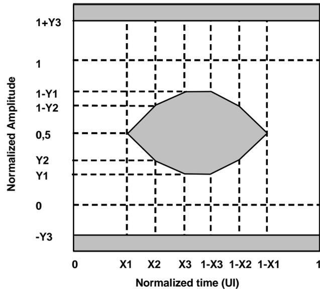
**Figure 21 – SM transmitter eye mask for 8GFC, and 16GFC**
