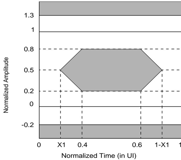
**Figure 20 – SM transmitter eye diagram mask for 4GFC**
