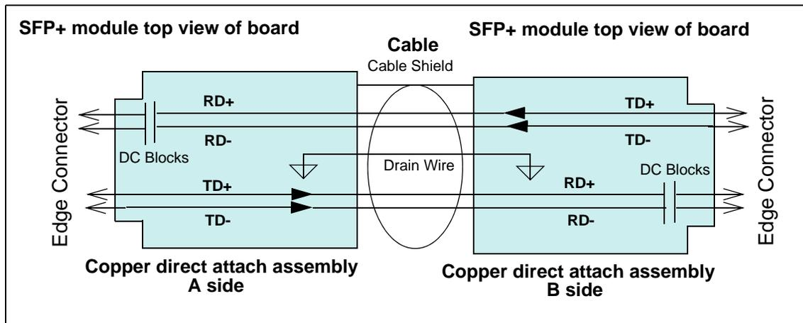
Figure C.1 – SFP+ direct attach block diagram
