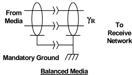
Figure 47 – Inter-enclosure receiver compliance point  $\gamma_R$
