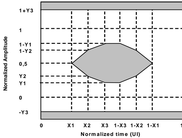
Figure 27 – MM transmitter eye mask for 8GFC and 16GFC
