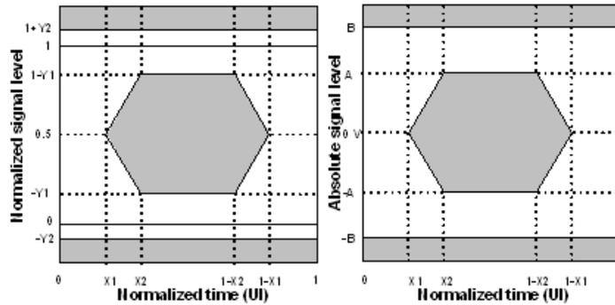
**Figure 40 – Normalized (left) and absolute (right) eye diagram masks at  $\beta_T$ ,  $\delta_T$  and  $\gamma_T$**
