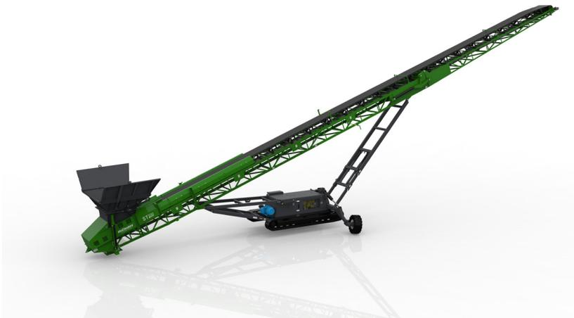
Hydraulic main lift and top fold are standard on the ST100TVR, as is the diesel power unit. Dual power is available to reduce operational costs and allow for remote location use, no matter what application. The 22.5 degree maximum conveyor angle allows for the highest stockpiles per conveyor length in the industry.
