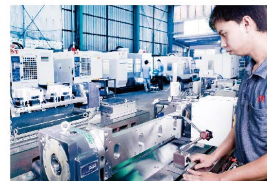
組裝前底板精度檢驗 ▲ Base plate accuracy inspection before assembling
